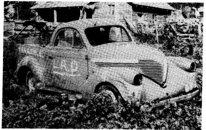
"Holden" bodied '37 Ute was based on their coupe body, had sloping roof, wing windows and split rear window.
