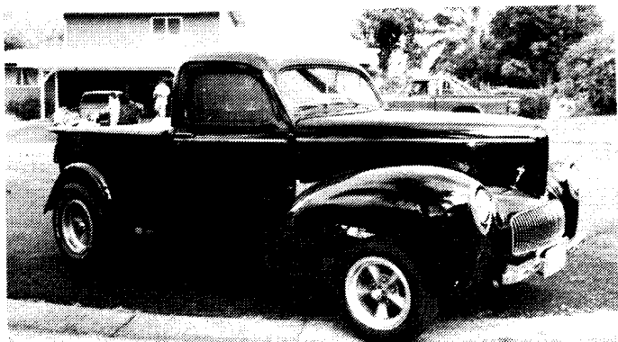
FRANK & BLAKE MEDEIROS, OLOMANA, OAHU. This tidy little pick-up runs a 283 Chevy powerplant with TH350 tranny, rear end is early Olds' with ladder bars. Paint is Black Ureglow, grille is hand made. American mags finish it off.
