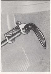
The emergency brake is conveniently located under the instrument panel. With pistol-grip, it can be grasped in an instant and quickly set. To release, merely turn the handle.
