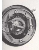
te big Bendix selfergizing brakes are nerously oversized. e same size and type brake used on cars ger and heavier than Willys provides an tra margin of safety.
