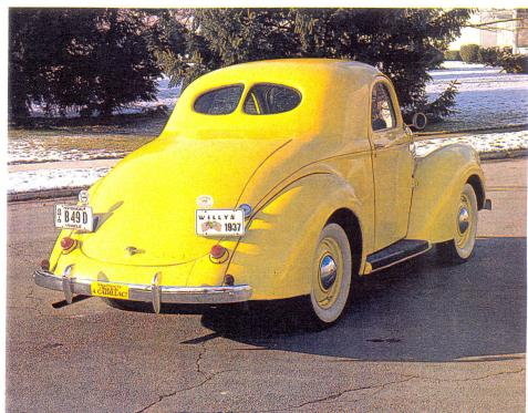
Although the Willys grew almost a foot to 175.5 inches for 1937 (both pages), the 100.5-inch wheelbase still measured a foot shorter than Chevrolet's. Its appearance was considered quite modern at the time, featuring smoothly curved, flowing lines with a gracefully rounded hood. The fenders were deeply crowned and the headlights were streamlined into their leading edges. (Owners: Ed and Eleanor Todd)
